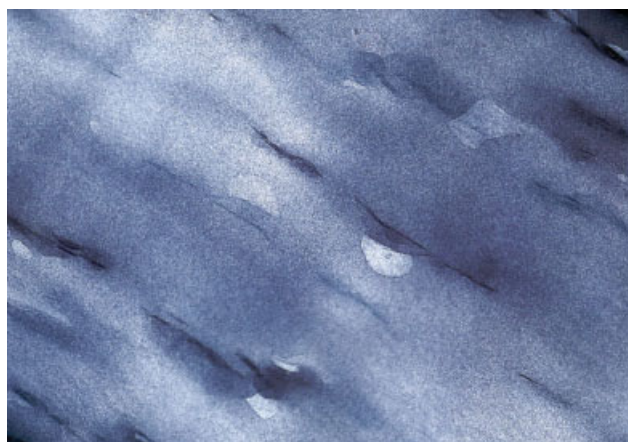
Figure 14 TEM micrograph on the core layer in the hybrid PE/PA6/clay film of “concentrated active layer” system—TPEcPac30. [Color figure can be viewed in the online issue, which is available at www.interscience.wiley.com .]
